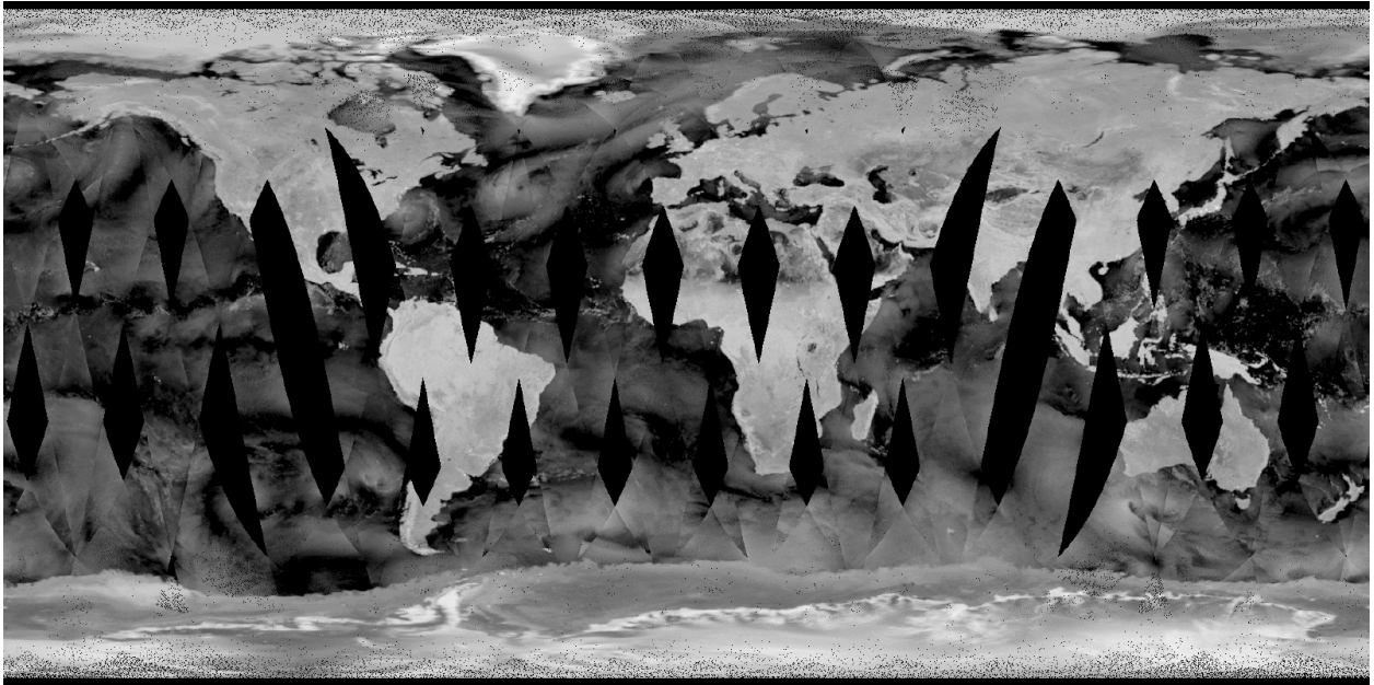
Figure 1: QS_XbhaG3C1999245.19992491643 (H-pol Global \sigma^0 browse image). Grey scale extends from -32 dB to 0 dB.
