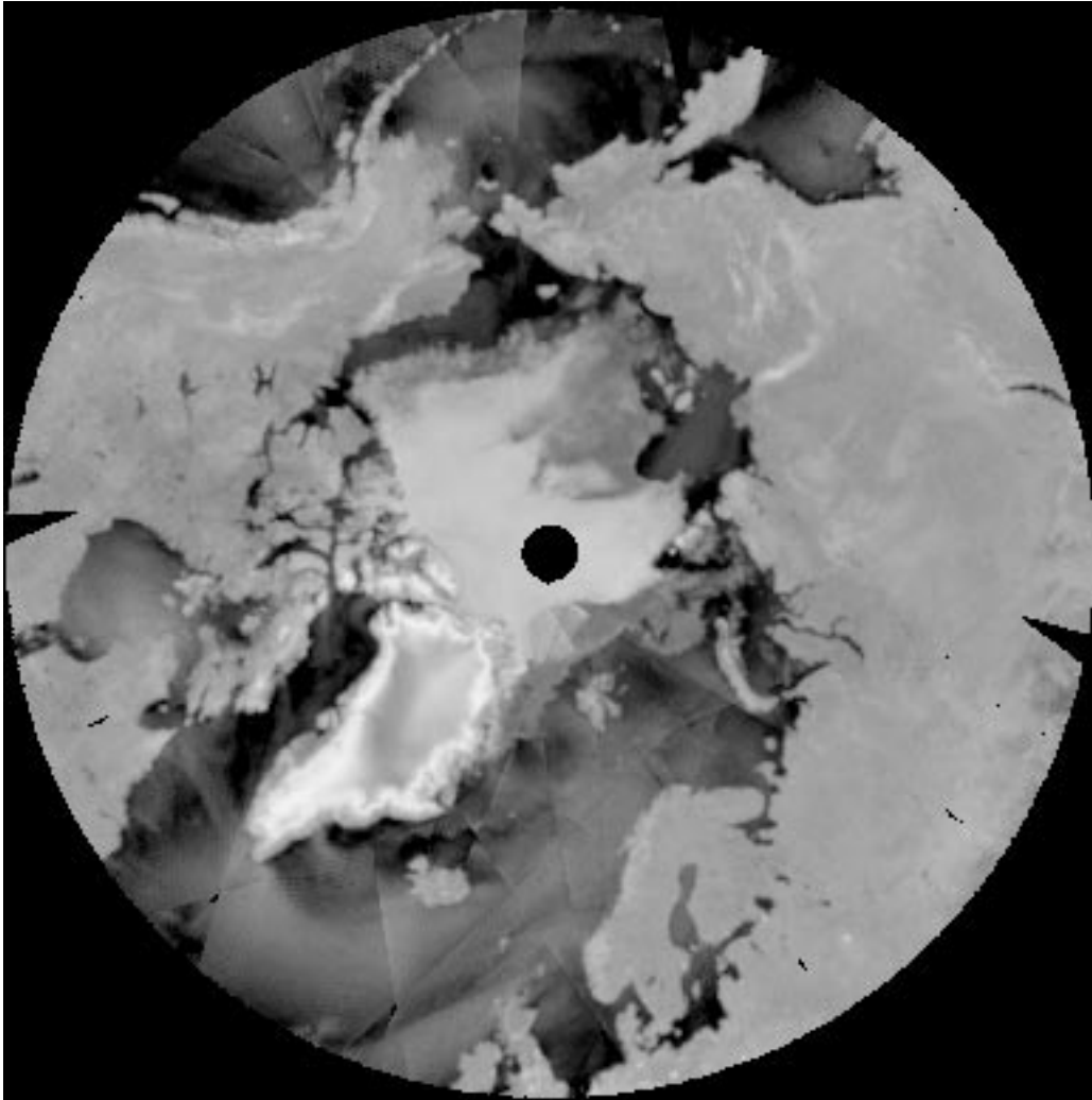
Figure 5: QS_XbhaN3C1999245.19992491643 (H-pol Northern Hemisphere \sigma^0 browse image). Grey scale extends from -32 to 0 dB.
