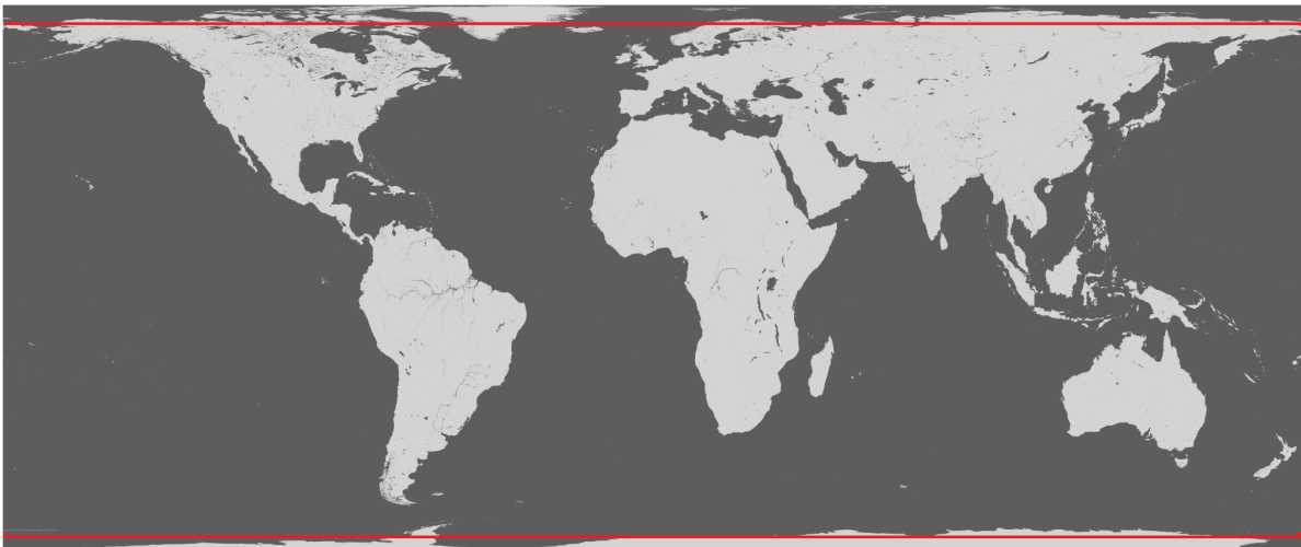
Figure 11: Cylindrical EASE-Grid 2.0 projection extents. Full extent coverage is EASE2-M, with horizontal red lines delineating the smaller latitudinal extent of EASE2-T grid. Land-ocean mask from Brodzik and Knowles (2011).
